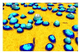
An example of a quantitative phase image of cells in 3D, created by HoloMonitor. The height of the cell and its color tone correspond to the optical thickness of the cell.
