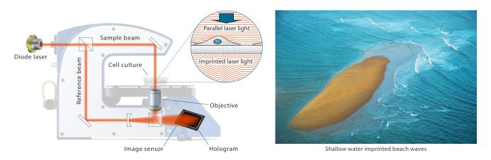
Holographic microscopy creates quantitative phase images by letting a sample beam and a reference beam interfere to create an interference pattern or *hologram*, as shown above. The hologram is recorded by an image sensor and computer processed to produce the phase image.
