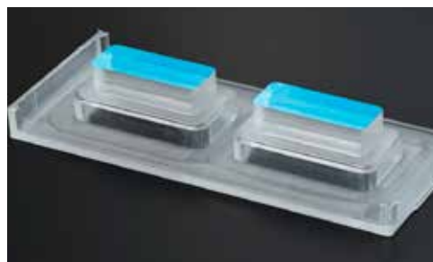
HoloLid placed in a Sarstedt 6-well plate (left). Note the cut edges in the left corner. The areas marked blue are the observation windows which are immersed into the cell media (right).
