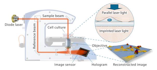
Holographic microscopy creates quantitative phase images by letting a sample beam and a reference beam interfere to generate an interference pattern – the hologram.
